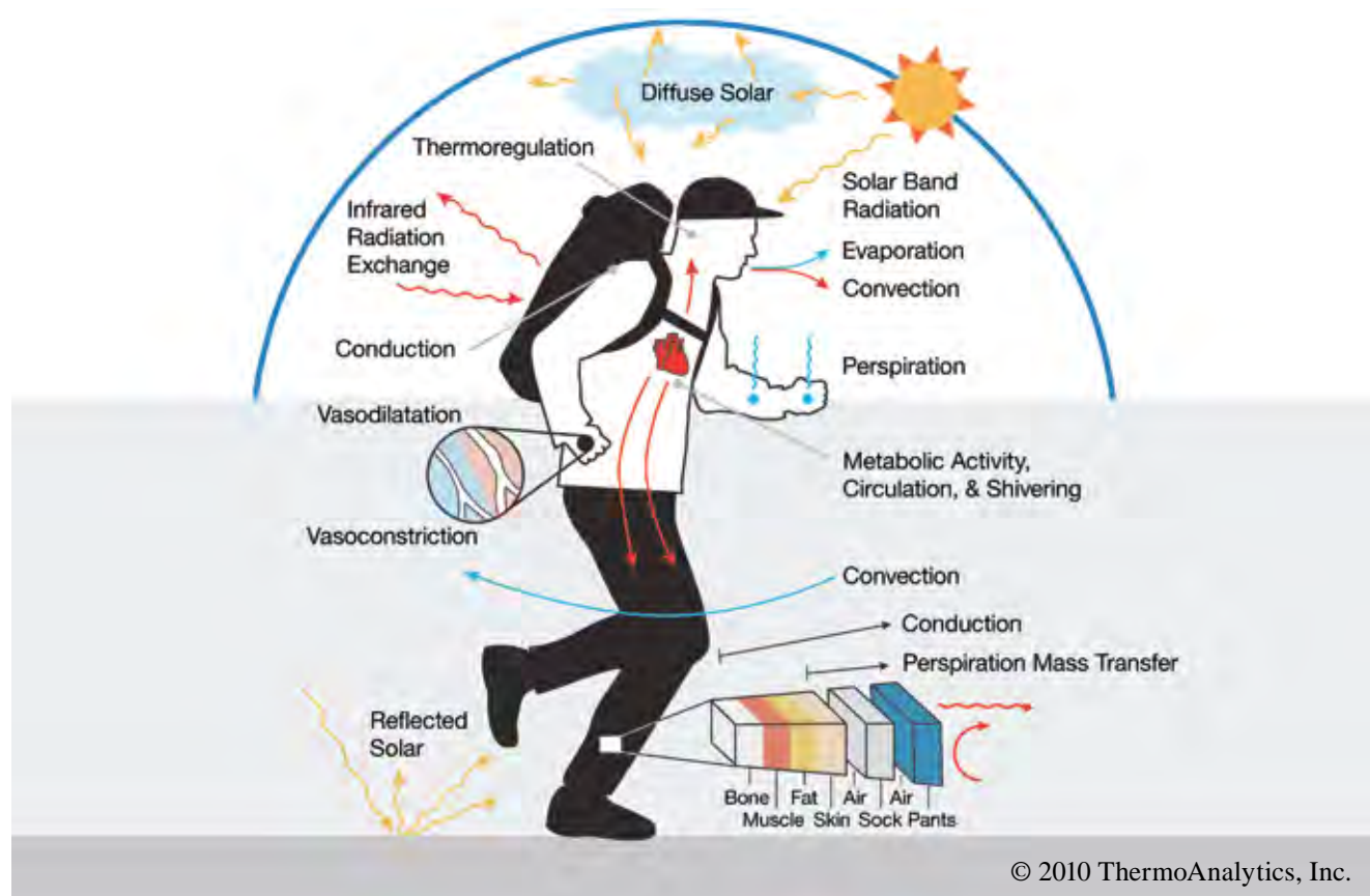
Figure 2.1: Temperature regulation. This diagram demonstrates the heat generated by internal processes (metabolism and muscle contraction) and the avenues of heat transfer to the surrounding environment (evaporation, radiation, conduction, convection).
