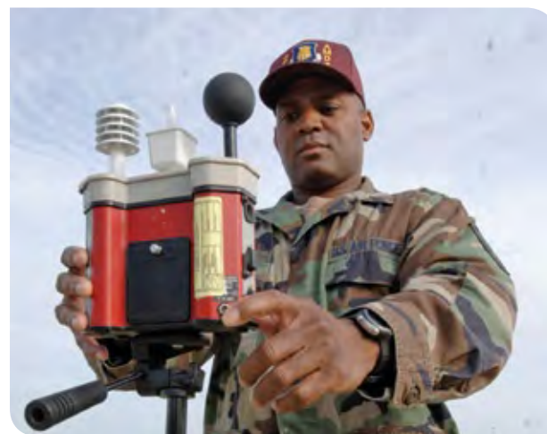
Figure 2.2: Measurement of the parameters comprising the Wet-Bulb Globe Temperature (WBGT) Index by military personnel. From left to right, the sensors are the dry-bulb thermometer ( T_{db} ), natural wet-bulb ( T_{wb} ) and the globe thermometer ( T_g ), which are incorporated by algorithm to represent the WBGT.
